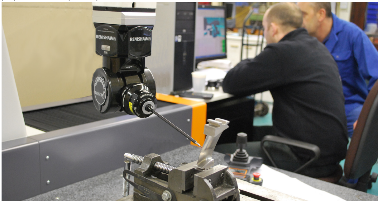
REVO five-axis measuring system inspecting a blade profile, including the previously un-measurable leading edge
