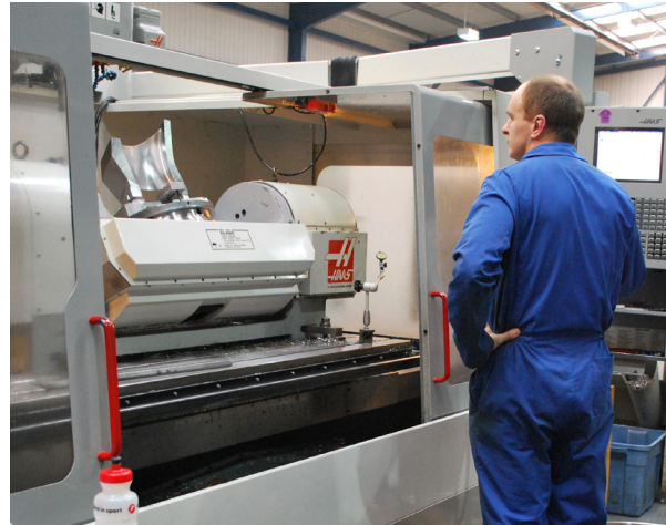
Parts with complex forms are produced on multi-axis machining centres
