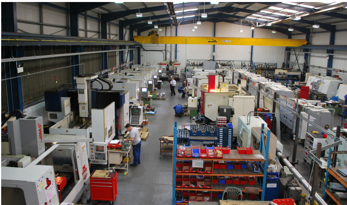
ANT's efficient machine shop includes multi-axis machining centres and turning centres equipped with touch probes
